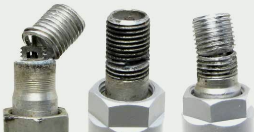
Galvanic corrosion causes TPMS failures
